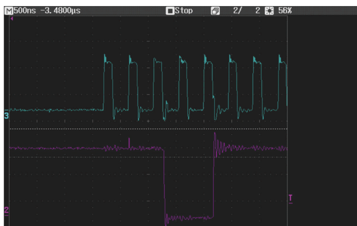
Figure 1 An IBIS simulation would be useful in this example, in which the clock- and data-signal-termination method creates signals that exceed specified high- and low-level thresholds. See the online version of this article at www.edn.com/100218bb for a block diagram of the system.
