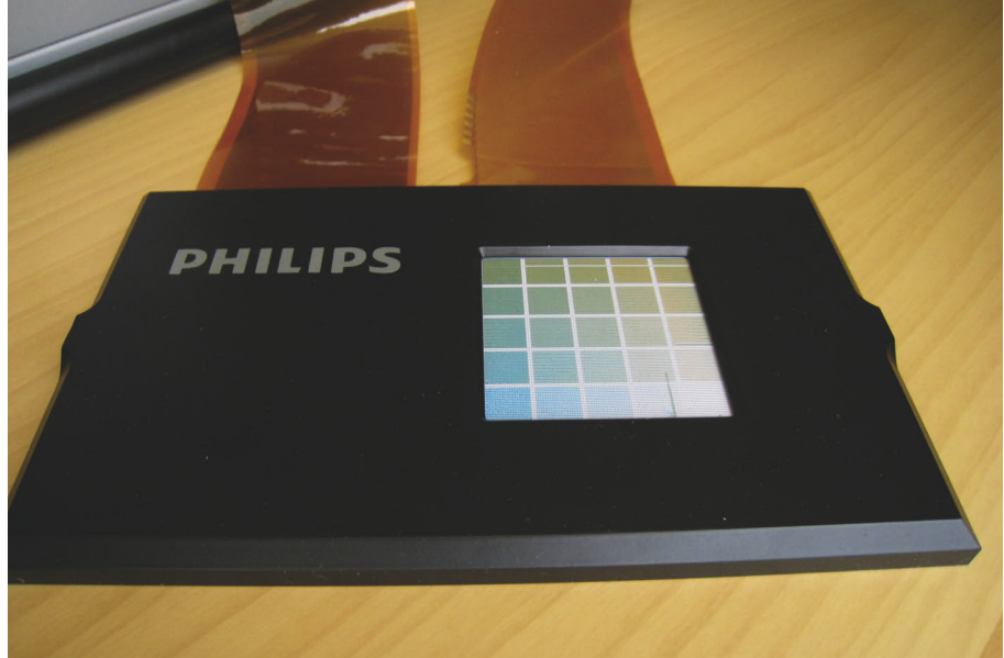
Philips' technology allows users to build different colors of ink into one layer and to control each color separately.
